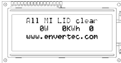
Upon completion of overall network unlocking communication between EVB201 and MI starts. On the first line of the LCD screen "x MI connected" shows how many MI units have been connected with "x" indicating the number of MIs connected. The second line indicates real-time power, today's energy production and the number of connected MIs, which all give "0" at this stage because the system is starting up. The third line presents the company website www.envertec.com (as shown below).
