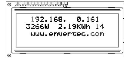
IP address shows on the first line. For example, 192.168.0.161\* indicates a normal network connection while 192.168.0.255 indicates no internet connection.
