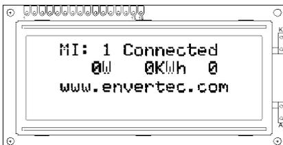
After the completion of network construction EVB201's start-up finishes and EVB201 enters normal working status. It will take a while before the monitoring interface shows up on the LCD screen. EVB201 will unlock and construct the network again automatically if there is a failure in network construction. The reconstruction of network will take place every 2 hours.
