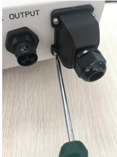
Fig. Dismantle the communication box
