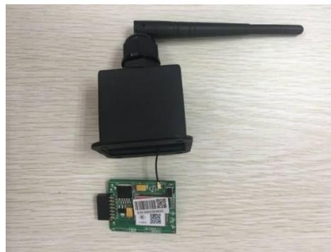
Fig. Connect the GPRS antenna
