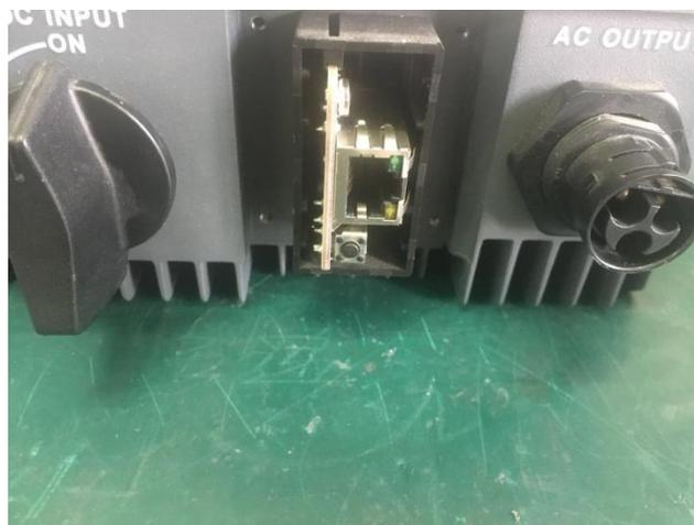
Connect the Ethernet cable to the Ethernet card.
