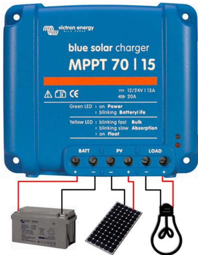
Figure 3: Power connections
